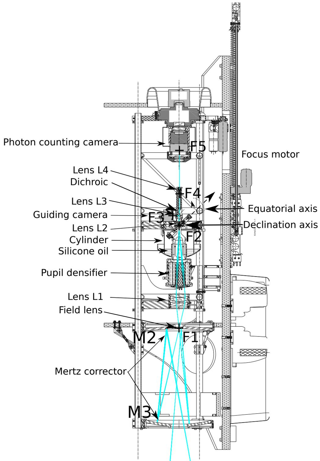
Figure 3. The focal module, attached to the carbon fiber tubes gondola presented Fig. 2, designed with the CATIA software. In blue, we have superimposed the optical rays computed with the Zemax software (see Fig. 4). F1 and F2 are respectively the Fizeau, and densified Focus. F3 and F5 are the densified foci magnified respectively for the guiding camera, and the photon counting camera.
