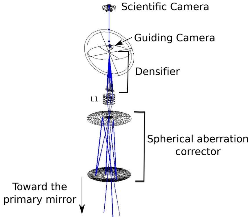
Figure 4. Optical design of the focal module computed with the Zemax software. On this view, we see the three beams coming from the three primary mirrors.
