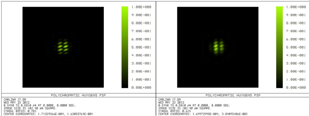
Figure 5. PSF (for the three mirrors of the OHP prototype), on axis (left) and off-axis by 0.15 arcsec (right) in the densified focal plane (F5 on Fig. 3) computed with the Zemax software.
